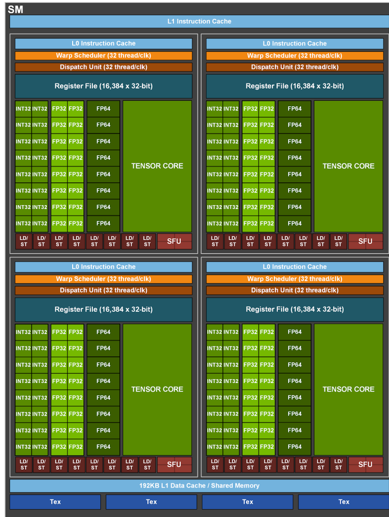
Figure 2.1: A single SM of an A100 GPU. Taken from an NVIDIA Blog Post 3
